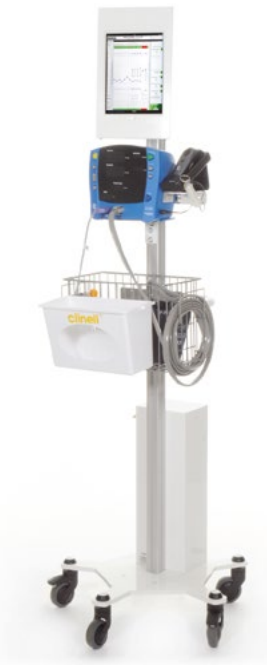
The SEND data entry hardware, comprising of a tablet, barcode scanner and bespoke roll stand capable of mounting most common vital signs monitors.
